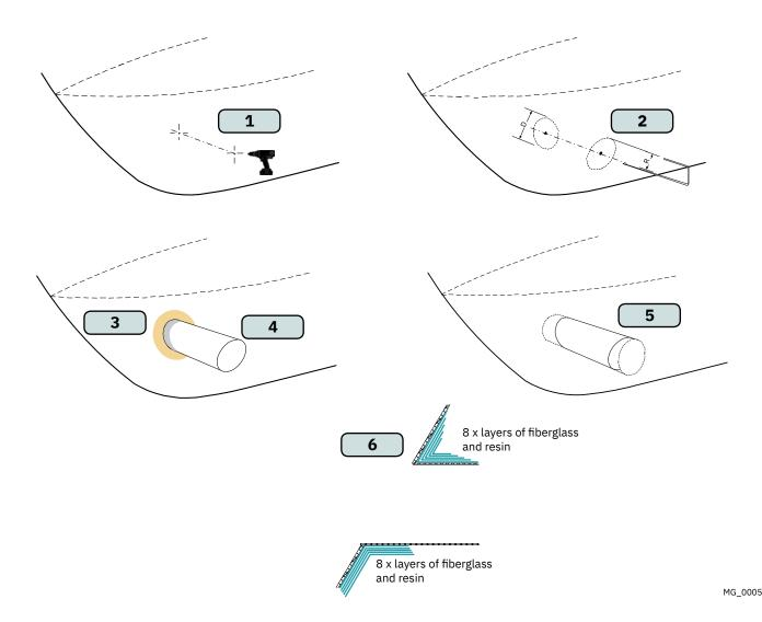
With tunnel installed and cast.
