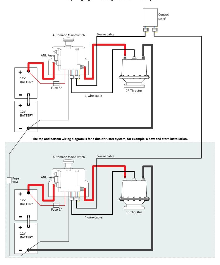
For **Control Panel** installation please refer to the Installation Guide accompanying the control panel to be installed.
