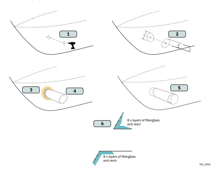
With tunnel installed and cast.
