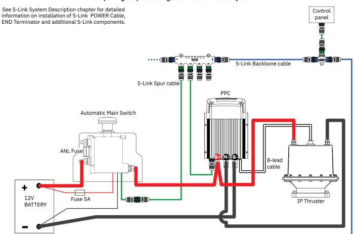
The top and bottom wiring setup is for a dual thruster system, For example bow and stern.
