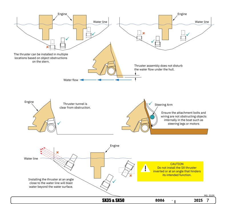
Sleipner cowls allow for increased flexibility in the thruster installation location.
