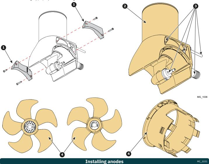
1. Re-install the anode on both sides of the gear housing. Note that the screws holding one anode has different lenghts, ensure using the correct screw. (**Reference 2**).
