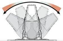
Variable thrust power for proportional thrusters is dependent on the extent of the joystick/ throttle.
